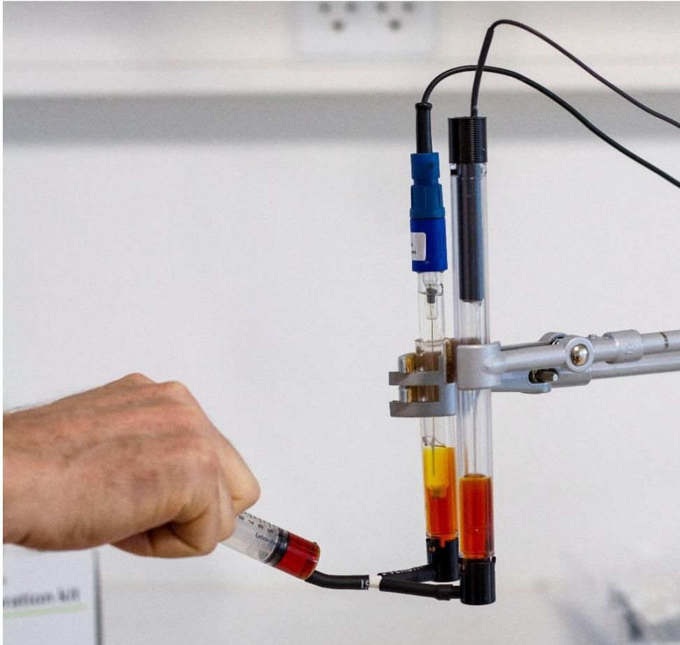
Figure 2: Redox electrode in the protection tube and reference electrode in the 10 cm transparent tube. The two Calibration Caps are mounted on the protection tubes and connected via the Y-connector. The redox calibration solution is injected using the 10 ml syringe.
